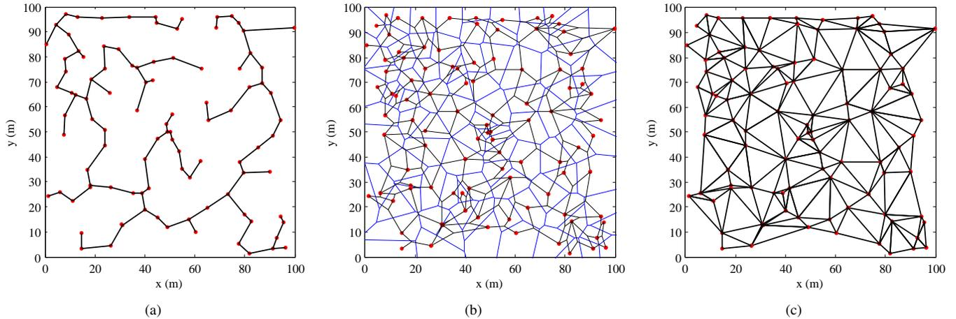
Fig. 6. The deployment results of (a) the MST algorithm, (b) the TC algorithm, and (c) the full-deployment strategy. (The red dots are the sensors; the black lines represent the MI waveguides; and the blue cells are the Voronoi diagrams. 100 sensors are uniformly distributed with a spatial intensity  $\lambda_{rand} = 0.01 \text{ m}^{-2}$ .)
