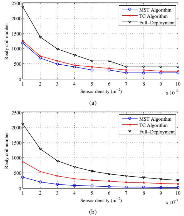
Fig. 5. The number of relay coils to connect 100 sensors in WUSNs with (a) hexagonal tessellation topology and (b) random topology.
