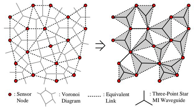
Fig. 4. The MI waveguide deployment using TC algorithm in the WUSN with random topology.
